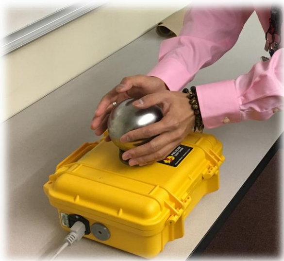
FIGURE 1. Demonstration of increased reactivity due to reflection using the reactivity simulator.
