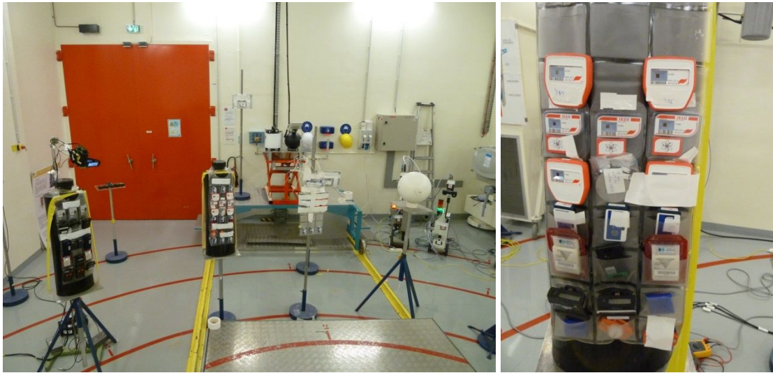
Figure 1 On the left, CALIBAN reactor – September 3rd experimental configuration; on the right, phantom with the different CADs.
